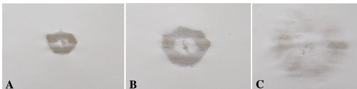
Figure 2. Spray Pattern Week 1. A. Formula 1 st with 3, 5 and 15 cm range of spray gel. B. Formula 2 nd with 3,5 and 15 cm range of spray gel. C. Formula 3 rd with 3, 5 and 15 cm range of spray gel.
