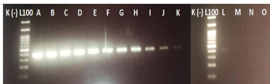
Figure 1. Electropherogram of E. coli PCR sensitivity test using serial dilution of E. coli DNA. The E. coli amplicon size is ± 417 bp. K(-): no template control; L100: DNA ladder 100 bp (Geneaid); A: DNA 10.15 ng/μL; B: DNA 5.08 ng/μL; C: DNA 2.54 ng/μL; D: DNA 1.27 ng/μL; E: DNA 0.63 ng/μL; F: DNA 0.32 ng/μL; G: DNA 0.16 ng/μL; H: DNA 0.08 ng/μL; I: DNA 0.04 ng/μL; J: DNA 0.02 ng/μL; K: DNA 0.01 ng/μL; L: DNA 0.005 ng/μL; M: DNA 0.0025 ng/μL; N: DNA 0.0013 ng/μL; O: DNA 0.0006 ng/μL.
