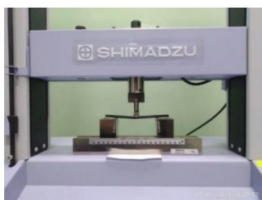
Gambar 1. Universal Testing Machine (UTM) 5 KN
